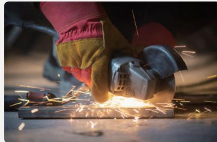
While operating a grinder, be very cautious not to overload it. If this happens, kickback can occur, throwing cut materials into the air or at the operator. When cutting objects placed on the floor, hold the grinder with the wheel facing inward to the left. By mastering the correct use of the grinder, you can protect yourself from potential hazards.
